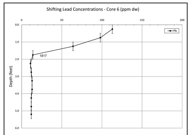
Figure 8. Trace element plot showing shifting concentrations of lead (Pb) for Core 6 in West Foundry Cove. Note uptick in lead levels between 1.25 and 1.75 ft. in depth. Chart by R.J. Taylor.
