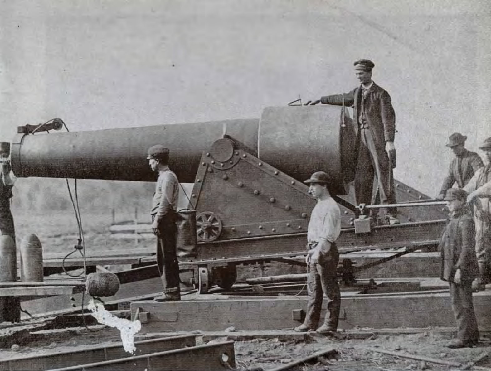
Civil War-era photo of gun crew testing R.P. Parrott's 30,000-pound rifled cannon. Children were often employed in the highly dangerous work. PUTNAM COUNTY HISTORICAL SOCIETY, NEW YORK
